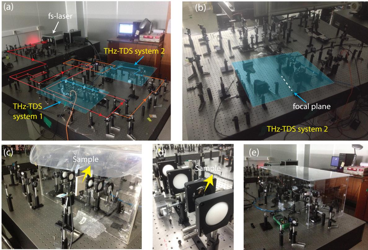
Figure 2.18: The constructed THz-TDS using (a) 4 Teflon lenses and (b) 4 parabolic mirrors, respectively. (c) The whole THz-TDS setup is purged with dry air to reduce the absorption by water vapor in the THz frequency range. (d) Enlarged sample section of THz-TDS in a linear configuration. (e) THz-TDS setup purged with acrylic box.
