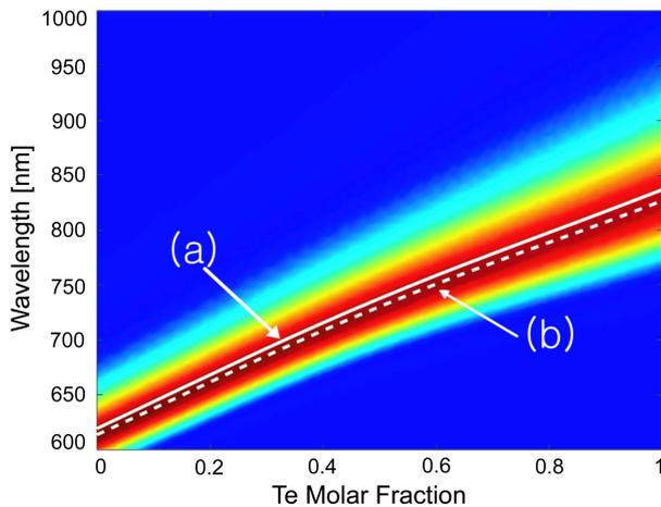
Fig. 4. Calculated total terahertz power from a 2-mm-thick  $\text{ZnSe}_{1-x}\text{Te}_x$  emitter, calculated with respect to the change in the pump laser's wavelength and the Te molar fraction. The solid line (a) is obtained when the momentum mismatch  $\Delta k$  becomes zero and the dashed line (b) is the total terahertz power maxima at a specific Te molar fraction.
