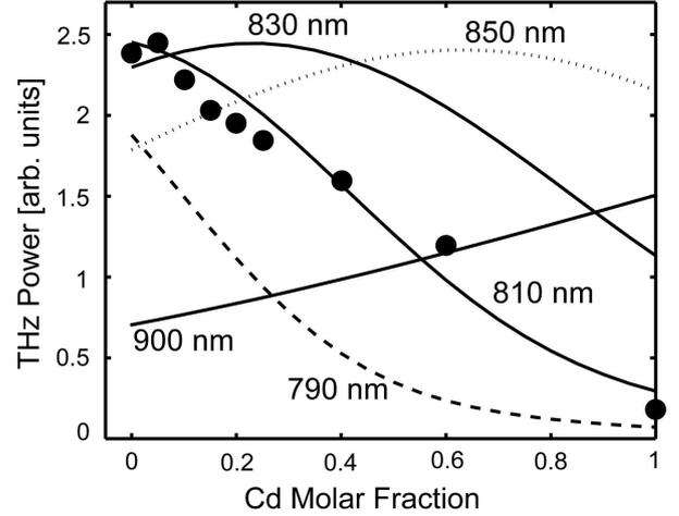
Fig. 3. Calculated terahertz power as a function Cd molar fraction for  $\text{Zn}_{1-x}\text{Cd}_x\text{Te}$  emitters. The wavelength of the ultrashort pump pulse is changed from 810 nm to 900 nm. The results of Liu *et al.* shown with filled circles [22] are comparable with the calculated power at a pump laser wavelength of 810 nm.
