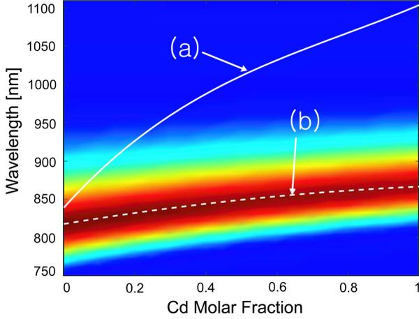
Fig. 2. Total terahertz power from a 2-mm-thick  $\text{Zn}_{1-x}\text{Cd}_x\text{Te}$  emitter, calculated with respect to the change in the pump laser is wavelength and the Cd molar fraction. The solid line (a) obtained from the condition that the momentum mismatch  $\Delta k$  becomes zero is different from the dashed line (b), the maxima of the terahertz power measured from the full calculation.
