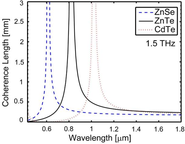
Fig. 1. Coherence length  $l_c(\lambda_{opt}; \Omega)$  measured at the generated terahertz frequency  $\Omega = 1.5$  THz as a function of the optical wavelength  $\lambda_{opt}$ . From left to right: ZnSe, ZnTe and CdTe.
